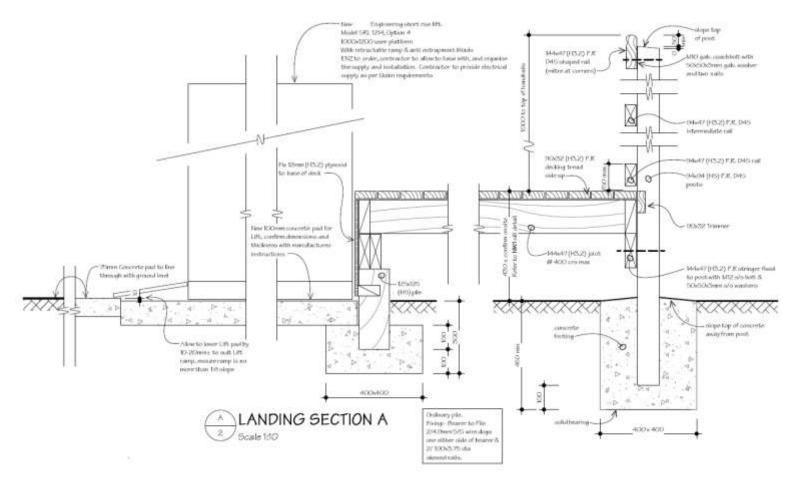
This is a <u>Sectional View</u> which is similar to an Elevation except it cuts through part of a building. Above is a sectional view of a ramp. It is as if it has been cut in half so you can see how it is actually put together. These views are part of the Working Drawings and are created so the council can see how something is going to be built and the contractor (or builder) can follow it when they come to building it.
