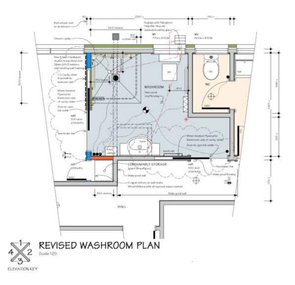
This is another <u>Plan View</u> but it is specific to a location. It show areas within the building in much more detail. This details the doors, more measurements, electrical wiring, fixtures and fittings.
