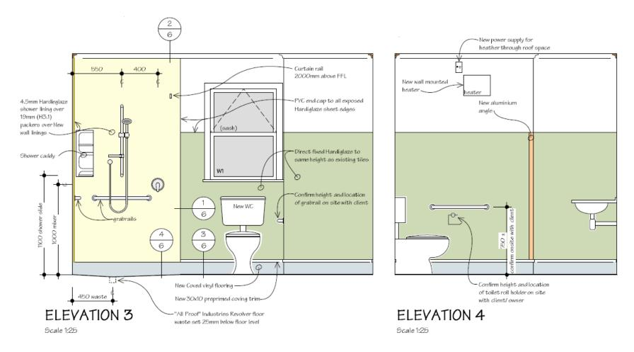
This is an <u>Elevation View</u> which shows a room or a whole house as if it were sliced down the middle. This is to give the viewer an impression of how the room will look per wall. The elevations will generally have a reference to them on one of the plan sheets. You will see from above that Elevation 4 is taken from the centre of the room with the window on your left shoulder. This is why the toilet is shown on Elevation 4 but the shower fittings are not.
