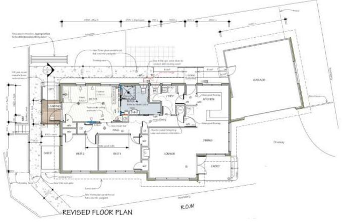
This is a <u>Plan view</u>. These views are from well above the building without the roof on so the wall and room layouts can be viewed.
